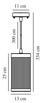
Voltage (V): 220-240 Volt IP degree: IP33 Maximum bulb wattage (W): 25W Class (Class 1, Class 2, Class 3): Class 2 (Double isolated) Socket type: E27 Parallel connection: True
