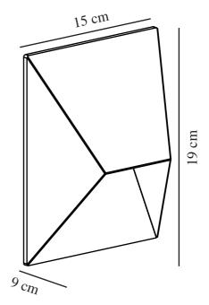
Voltage (V): 220-240 Volt IP degree: IP54 Maximum bulb wattage (W): 25W Class (Class 1, Class 2, Class 3): Class 1 (Earth contact) Socket type: GU10 Parallel connection: True
