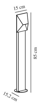
Voltage (V): 220-240 Volt IP degree: IP54 Maximum bulb wattage (W): 25W Class (Class 1, Class 2, Class 3): Class 1 (Earth contact) Socket type: GU10 Parallel connection: True
