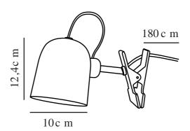
Voltage (V): 220-240 Volt IP degree: IP20 Maximum bulb wattage (W): 15W Class (Class 1, Class 2, Class 3): Class 2 (Double isolated) Socket type: GU10 Switch placement: On the cable
