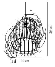
Voltage (V): 230 Volt IP degree: IP20 Maximum bulb wattage (W): 60W Class (Class 1, Class 2, Class 3): Class 2 (Double isolated) Socket type: E27 Dimmerable: Yes with compatible bulb
