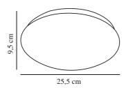
Voltage (V): 230 Volt IP degree: IP20 Class (Class 1, Class 2, Class 3): Class 1 (Earth contact) Socket type: LED Module
