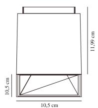
Voltage (V): 230 Volt IP degree: IP20 Maximum bulb wattage (W): 50W Class (Class 1, Class 2, Class 3): Class 2 (Double isolated) Socket type: GU10 Parallel connection: True
