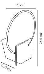
Voltage (V): 230 Volt IP degree: IP44 Class (Class 1, Class 2, Class 3): Class 2 (Double isolated) Socket type: LED Module
