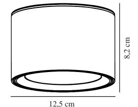
Voltage (V): 220-240 Volt IP degree: IP44 Class (Class 1, Class 2, Class 3): Class 2 (Double isolated) Socket type: LED Module Parallel connection: True
