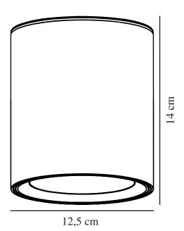
Voltage (V): 220-240 Volt IP degree: IP44 Class (Class 1, Class 2, Class 3): Class 2 (Double isolated) Socket type: LED Module Parallel connection: True
