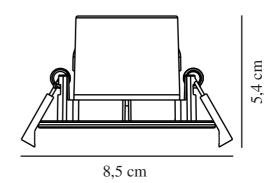
Voltage (V): 220-240 Volt IP degree: IP65 Class (Class 1, Class 2, Class 3): Class 2 (Double isolated) Socket type: LED Module Parallel connection: True
