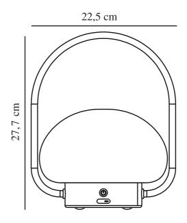
Voltage (V): 5 Volt IP degree: IP65 Class (Class 1, Class 2, Class 3): Class 3 (12V) Socket type: LED Module
