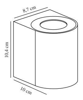
Voltage (V): 230 Volt IP degree: IP44 Class (Class 1, Class 2, Class 3): Class 1 (Earth contact) Socket type: LED Module Dimmerable: False Parallel connection: True
