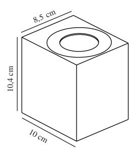
Voltage (V): 230 Volt IP degree: IP44 Class (Class 1, Class 2, Class 3): Class 1 (Earth contact) Socket type: LED Module Dimmerable: False Parallel connection: True
