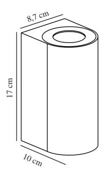
Voltage (V): 230 Volt IP degree: IP44 Maximum bulb wattage (W): 2X28W
