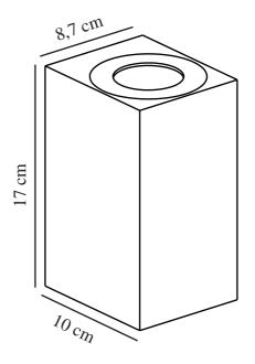
Voltage (V): 230 Volt IP degree: IP44 Maximum bulb wattage (W): 2X28W Class (Class 1, Class 2, Class 3): Class 1 (Earth contact) Socket type: GU10 Parallel connection: True
