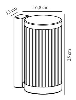
Voltage (V): 220-240 Volt IP degree: IP54 Maximum bulb wattage (W): 25W Class (Class 1, Class 2, Class 3): Class 1 (Earth contact) Socket type: E27 Parallel connection: True
