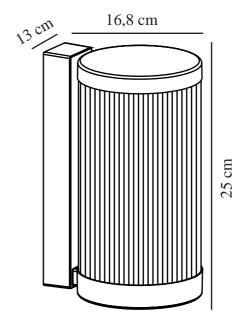
Voltage (V): 220-240 Volt IP degree: IP54 Maximum bulb wattage (W): 25W Class (Class 1, Class 2, Class 3): Class 1 (Earth contact)
