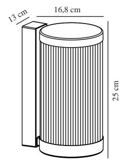
Voltage (V): 220-240 Volt IP degree: IP54
