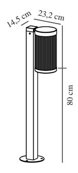
Voltage (V): 220-240 Volt IP degree: IP54
