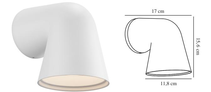
Voltage (V): 230 Volt IP degree: IP44 Maximum bulb wattage (W): 28W Class (Class 1, Class 2, Class 3): Class 1 (Earth contact) Socket type: GU10 Parallel connection: True
