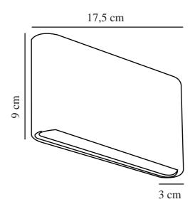
Voltage (V): 220-240 Volt IP degree: IP54 Class (Class 1, Class 2, Class 3): Class 1 (Earth contact) Socket type: LED Module
