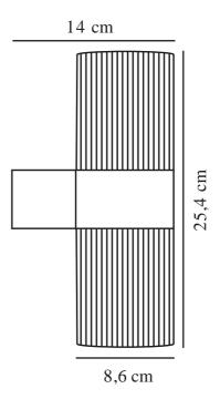
Voltage (V): 220-240 Volt IP degree: IP54 Maximum bulb wattage (W): 2x25W Class (Class 1, Class 2, Class 3): Class 1 (Earth contact) Socket type: GU10 Parallel connection: True
