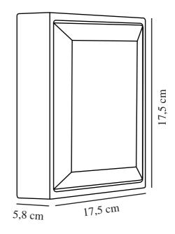
Voltage (V): 220-240 Volt IP degree: IP54 Class (Class 1, Class 2, Class 3): Class 2 (Double isolated) Socket type: LED Module Parallel connection: False
