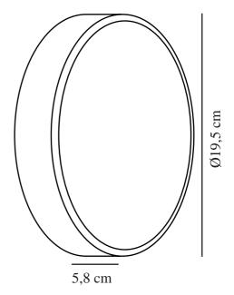
Voltage (V): 220-240 Volt IP degree: IP54
