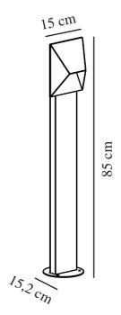
Voltage (V): 220-240 Volt IP degree: IP54
