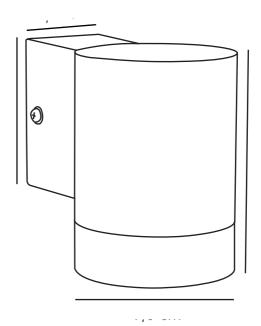
Voltage (V): 230 Volt IP degree: IP54 Maximum bulb wattage (W): 35W Class (Class 1, Class 2, Class 3): Class 1 (Earth contact) Socket type: GU10 Parallel connection: False
