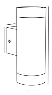
Voltage (V): 230 Volt IP degree: IP54 Maximum bulb wattage (W): 2X35W
