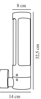
Voltage (V): 230 Volt IP degree: IP44 Maximum bulb wattage (W): 8W Class (Class 1, Class 2, Class 3): Class 1 (Earth contact) Socket type: GU10
