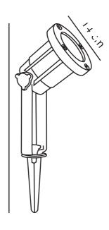
Voltage (V): 230 Volt IP degree: IP54 Maximum bulb wattage (W): 35W Class (Class 1, Class 2, Class 3): Class 1 (Earth contact) Socket type: GU10 Parallel connection: False
