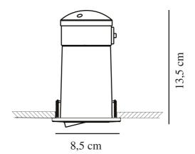
Voltage (V): 230 Volt IP degree: IP23 Maximum bulb wattage (W
