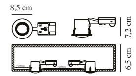
Voltage (V): 230 Volt IP degree: IP23 Maximum bulb wattage (W): 8W
