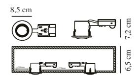
Voltage (V): 230 Volt IP degree: IP23 Maximum bulb wattage (W): 8W LED Class (Class 1, Class 2, Class 3):
