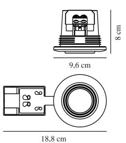
Voltage (V): 220-240 Volt IP degree: IP44 Maximum bulb wattage (W): 7,5W LED Class (Class 1, Class 2, Class 3): Class 2 (Double isolated) Socket type: GU10 Parallel connection: True
