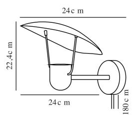
Voltage (V): 220-240 Volt IP degree: IP20 Maximum bulb wattage (W): 40 Class (Class 1, Class 2, Class 3): Class 2 (Double isolated) Socket type: GU10 Switch placement: On the base Parallel connection: False
