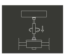
Step 2 Taking care not to damage any house wiring, detach the mounting strap from the fitting and affix to the ceiling using the screws supplied.
