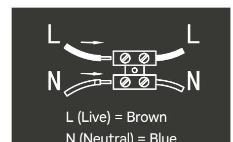
Check that you have correctly identified the house wires, that all connections are tight, and that no loose strands have been left out of the connection blocks.
