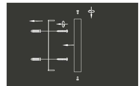
These screws should penetrate the joist by at least 2cm.
