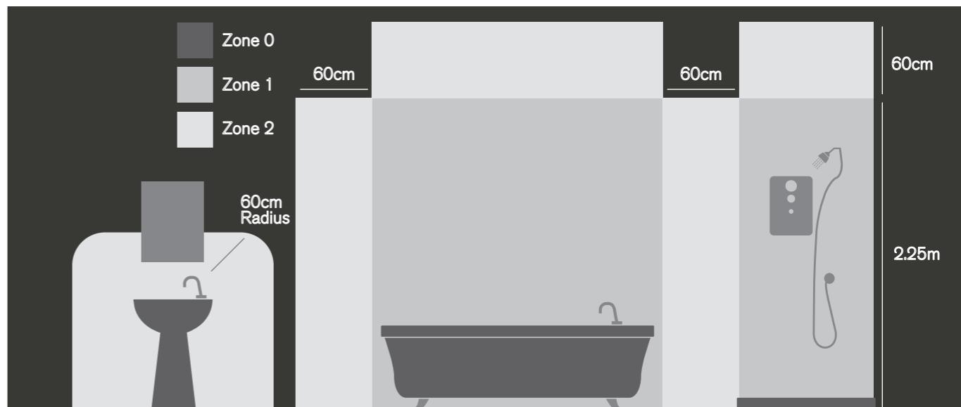
This product is rated IP44 and is suitable for installation in ZONE 2 and the area outside the zones. It can also be installed in ZONE 1 if connected to a 30mA RCD protected circuit.
