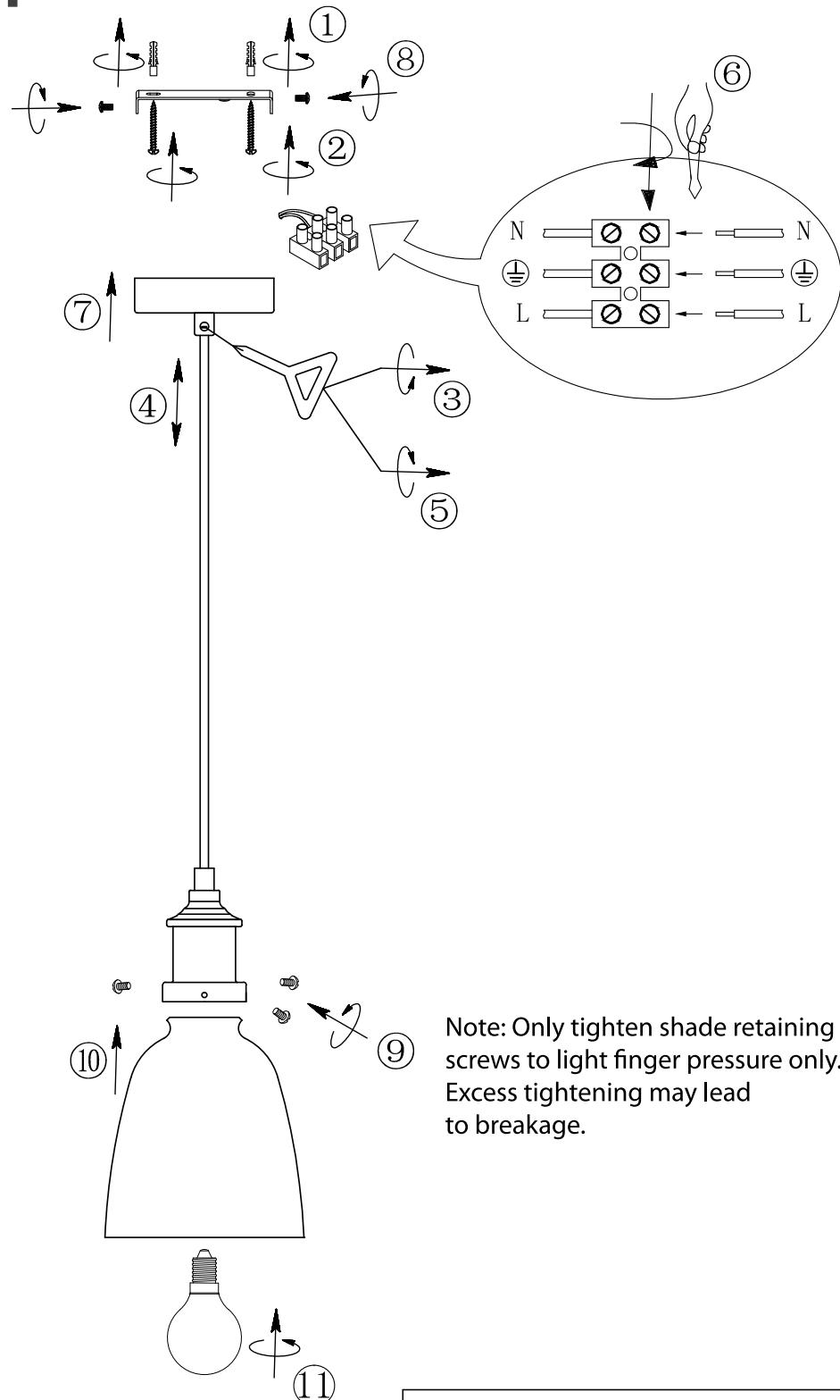
Note: Only tighten shade retaining screws to light finger pressure only. Excess tightening may lead to breakage.
